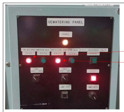
Fwd void space and Bosun store valve for driving the eductor are remotely controlled from the panel on bridge and are kept shut, these are opened only during pumping out of the water.
